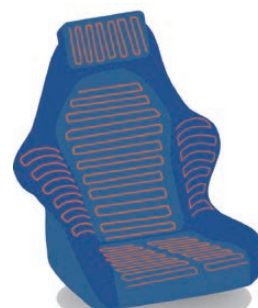
Heater wires sewn into a seat
